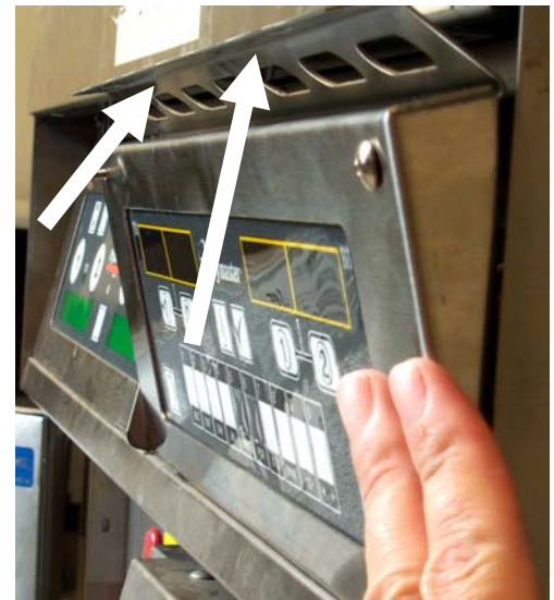
Figure 11: Rotate the computer into place. Secure to fryer at the top of the bezel. Use screws which held in the original computer. See arrows above.
