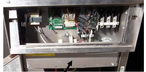
Figure 5: Locate and remove the plate covering the lower portion of the controller box. See arrow.
