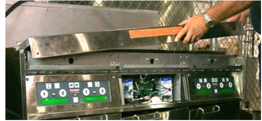
Figure 1: Remove top cap to gain access to mounting point for new speaker.
